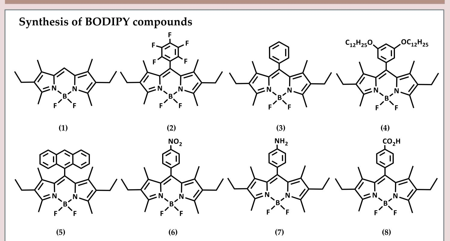
BODIPY's were prepared through the condensation of the correspondent aldehyde with two mono a-free pyrroles, leading to the formation of a dipyrromethane which was oxidized to dipyrromethene by 2,3-dichloro-5,6-dicyano-1,4-benzoquinone and, finally, complexed with boron by addition of BF<sub>3</sub>.Et<sub>2</sub>O in the presence of triethylamine.
