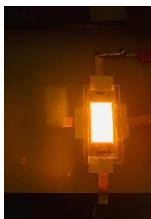
Figure 4. Image of 28mm by 50 mm OLED
